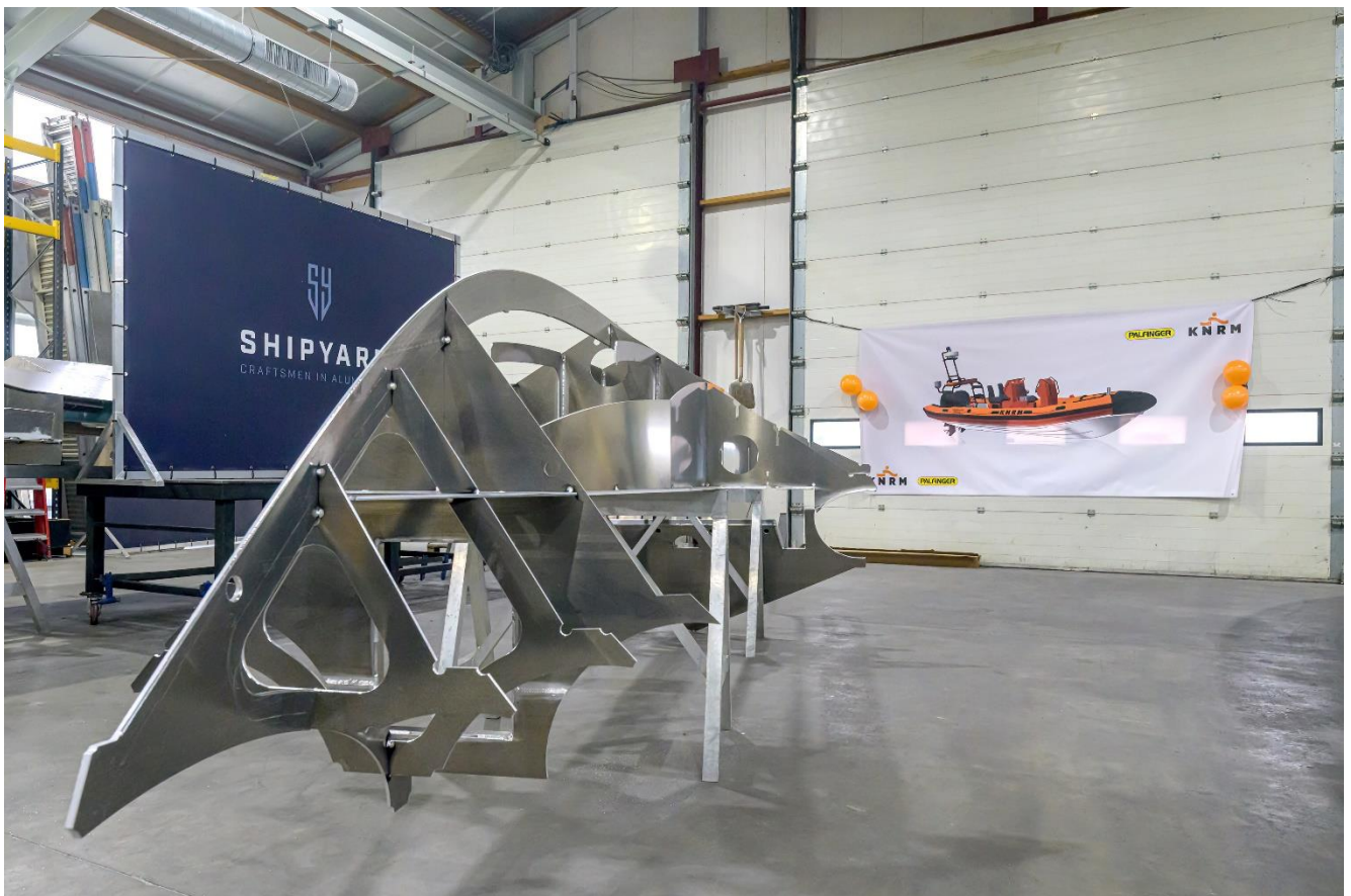
The keel of the rescue boat prototype in Dronrijp, the Netherlands, where the robust hull of the first prototype will be produced. © KNRM / Roel Ovinge Photography
